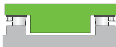
Vibration insulation concrete block or steel platform
